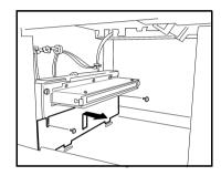
4 Remove the front and rear Shield Plate. (loosen the four screws)
